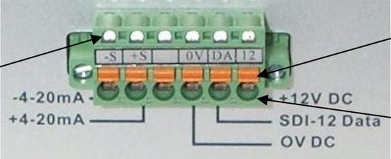
Multimeter probe can be inserted here !!!
