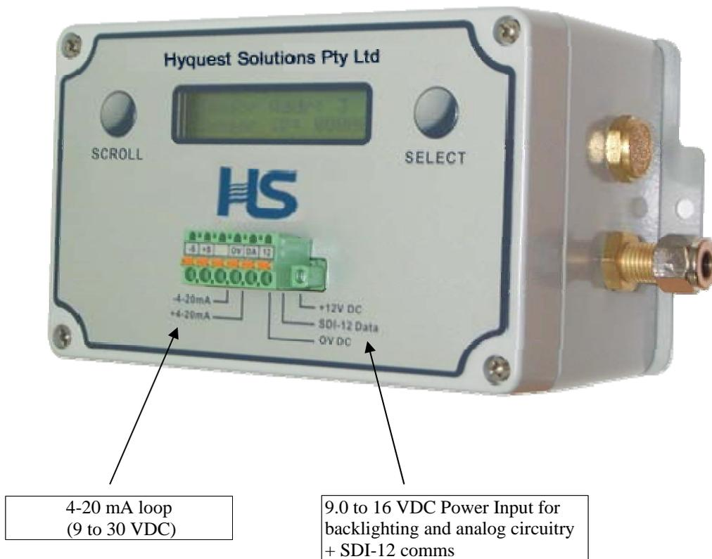
Figure5: External Power Connections
