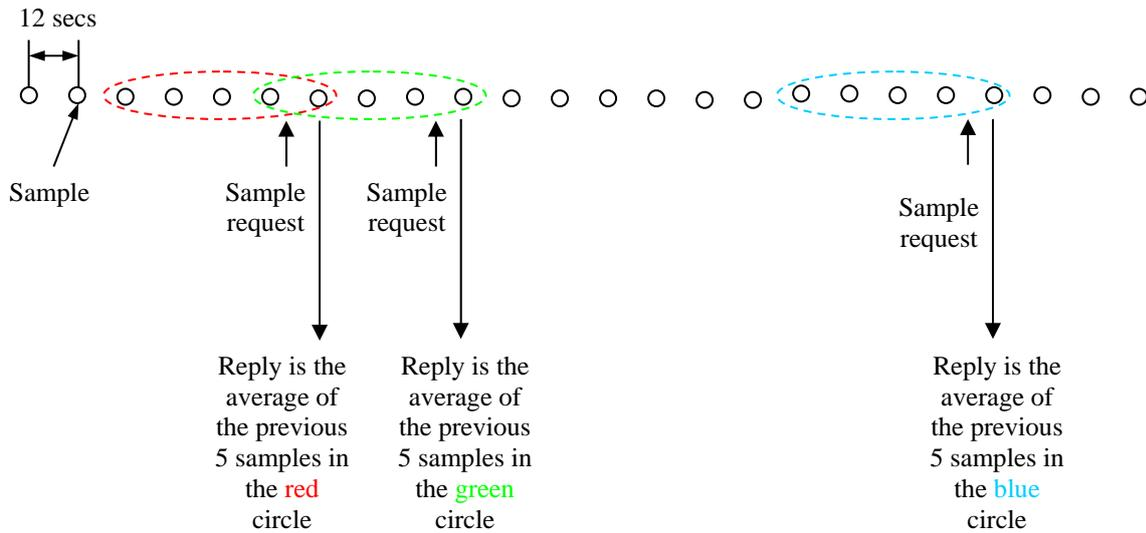
When a sample is requested (via the LCD, SDI-12 M command or 4-20mA), the next periodic sample will reply with an average of the previous 5 samples (obviously the number of samples used to calculate the average will depend upon the setting selected - between 1 and 20).
