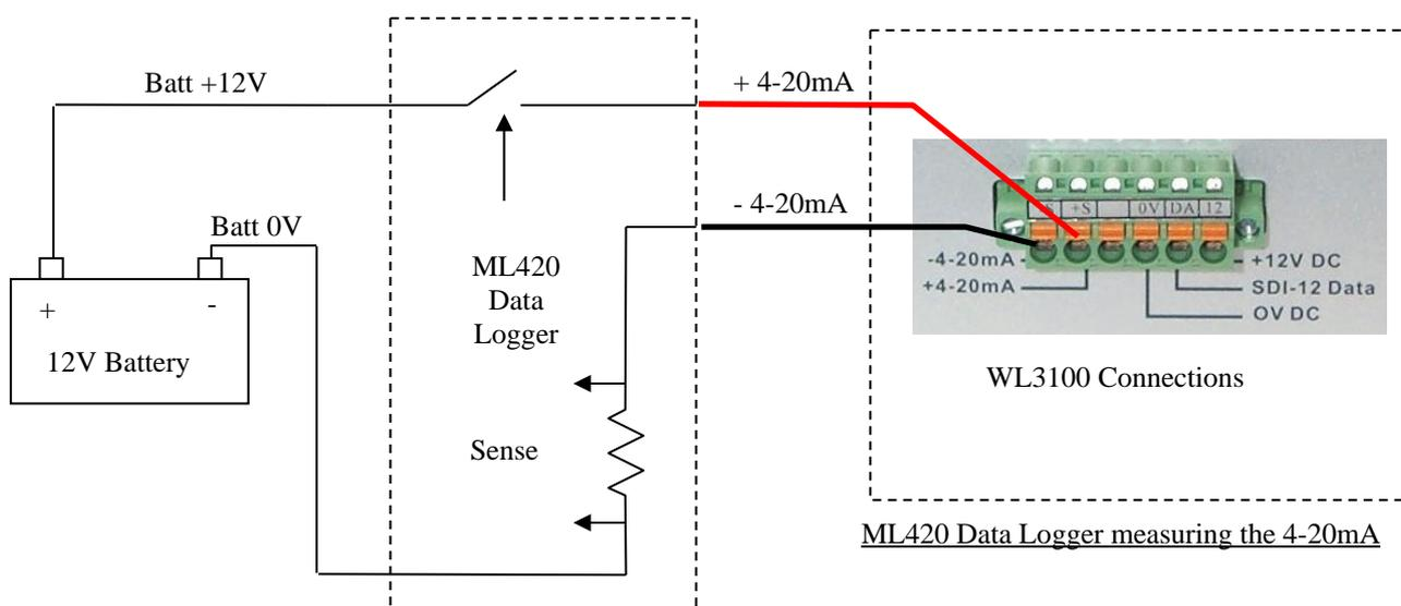
To conserve power, the data logger switches power to the 4-20mA circuit only when it wants to make a measurement.
