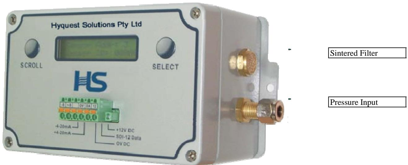
**Note: All units are factory calibrated over their full operating temperature and pressure range in our Environmental Chamber and Ruska Pressure Calibrator. A calibration certificate is supplied with each Sensor.**
