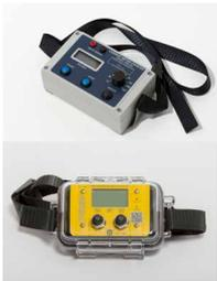
**Current Meter Counters** (various models): Features: waterproof enclosures, simple button controlled menus, embedded LCDs and beepers to make counts audible. Pre-set
