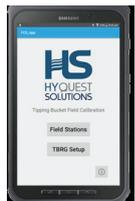
**FCD-App:** The FCD-App is free software developed and supported by HyQuest Solutions. It provides the most accurate and comfortable way for collecting data when performing a field calibration of a tipping bucket rain gauge. The app operates on any Android platform (customer's own tablet or phone) with bluetooth technology. The App is used in combination with HyQuest Solutions' counter CMCbt.
