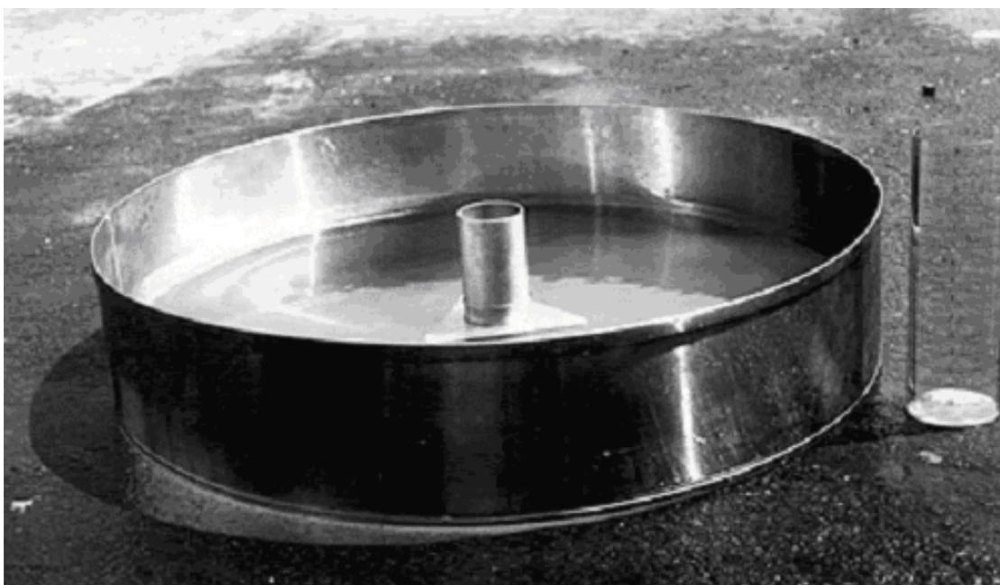
**Figure 1:** CLASS A EVAPORATION PAN WITH FIXED POINT GAUGE AND MEASURING CYLINDER
