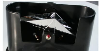
**Long-life pivots/bearings:** The new Series II models feature field-proven high-quality sapphire pivots. Sapphire is a stone and subsequently free from corrosion. Additionally, sapphires do not show any traces of wear and tear from bucket tips. This further extends the lifespan of the TB4 and the TB6 Series II.
